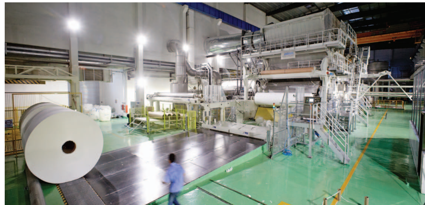
▲ The two new PrimeLine ™ tissue machines are equipped with the latest resource-saving technologies: the PrimeDry Steel Yankee and the ReEvaporation system.
