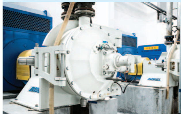
◀ ANDRITZ Double Disc TwinFlo Refiner for optimum fiber development.
