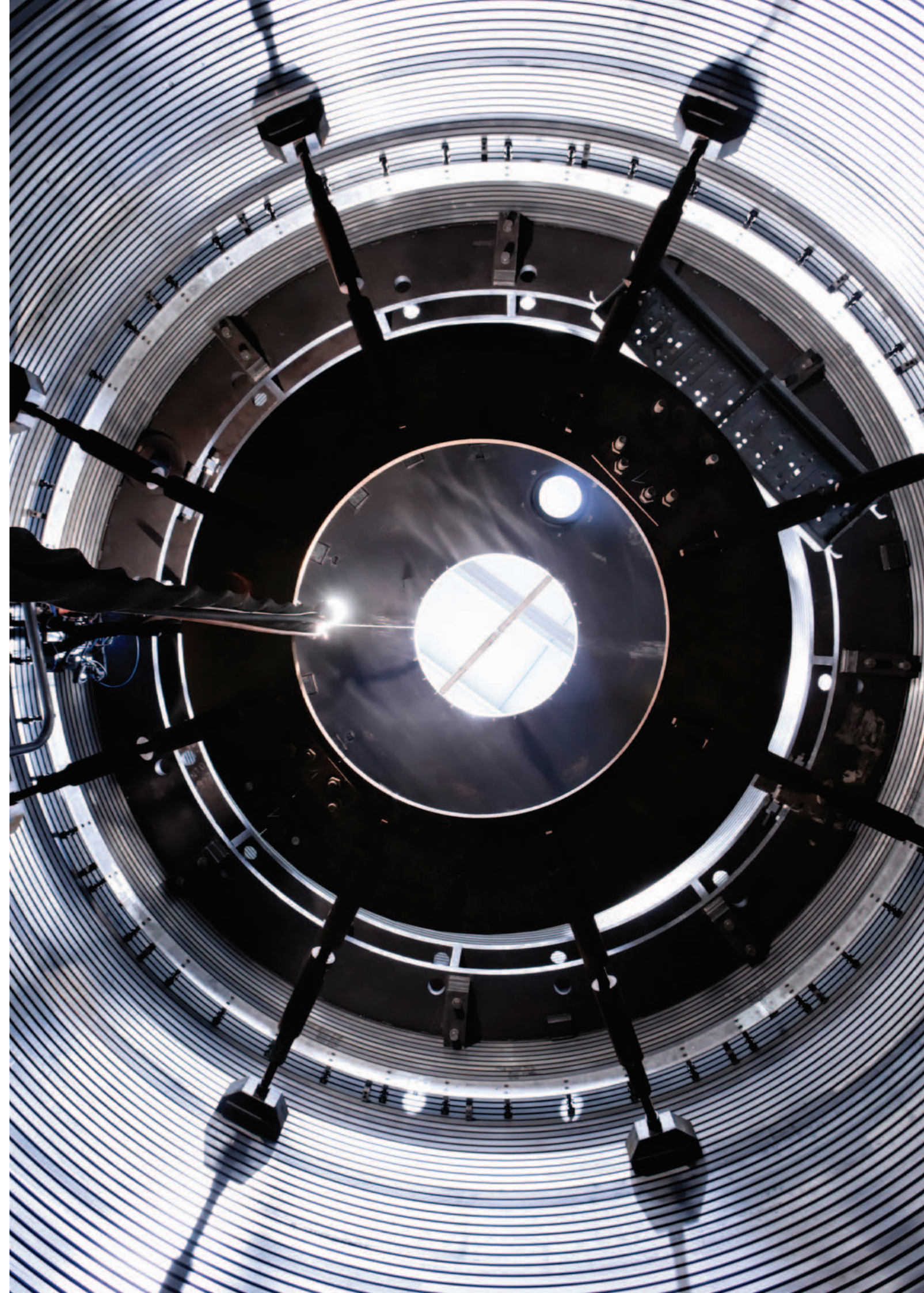
Inner view of a steel Yankee. ▶
