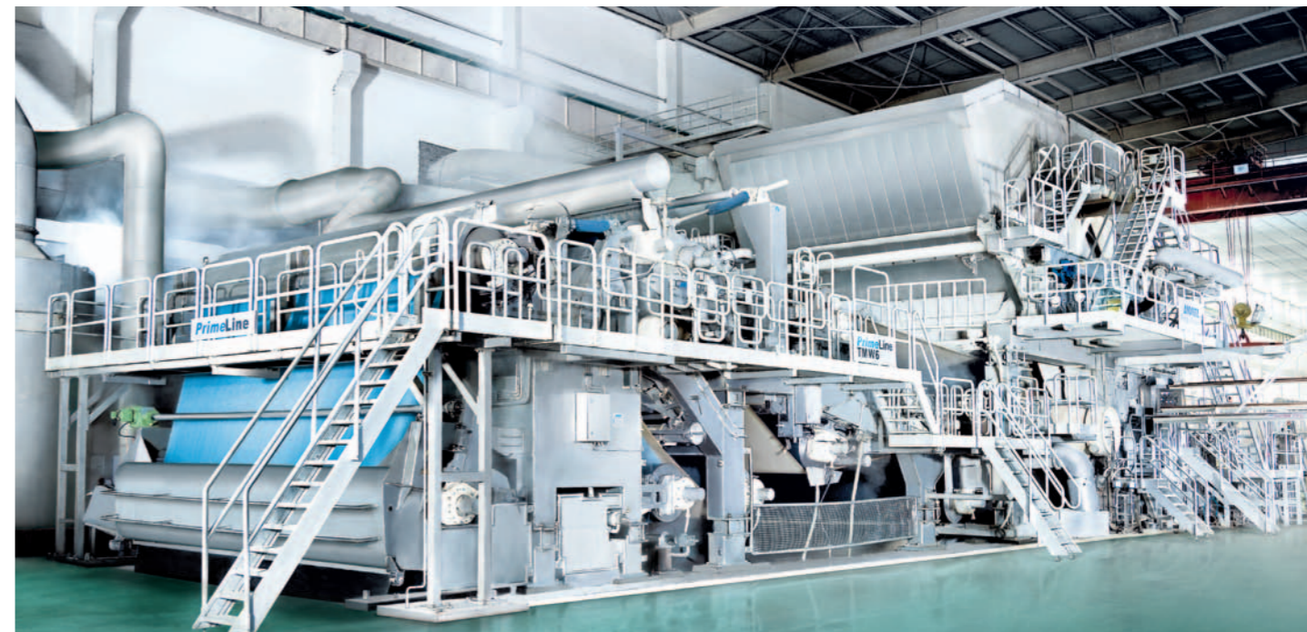
▲ Hengan's PrimeLineTM machines are equipped with the latest resource-saving technologies: the PrimeDry Steel Yankee and the ReEvaporation system.
