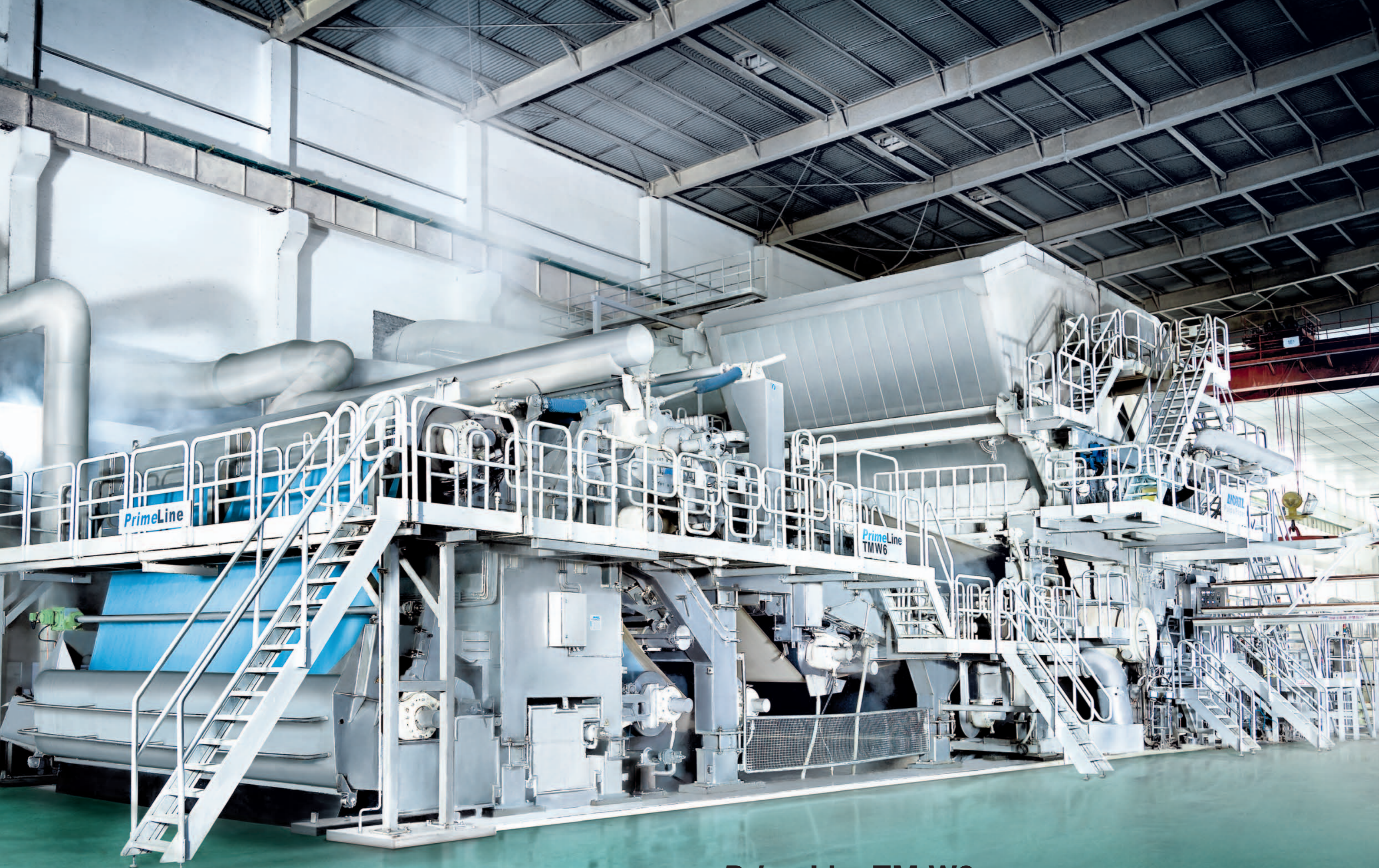
PrimeLine TM W8 High-speed tissue machine with 5.6 m width
