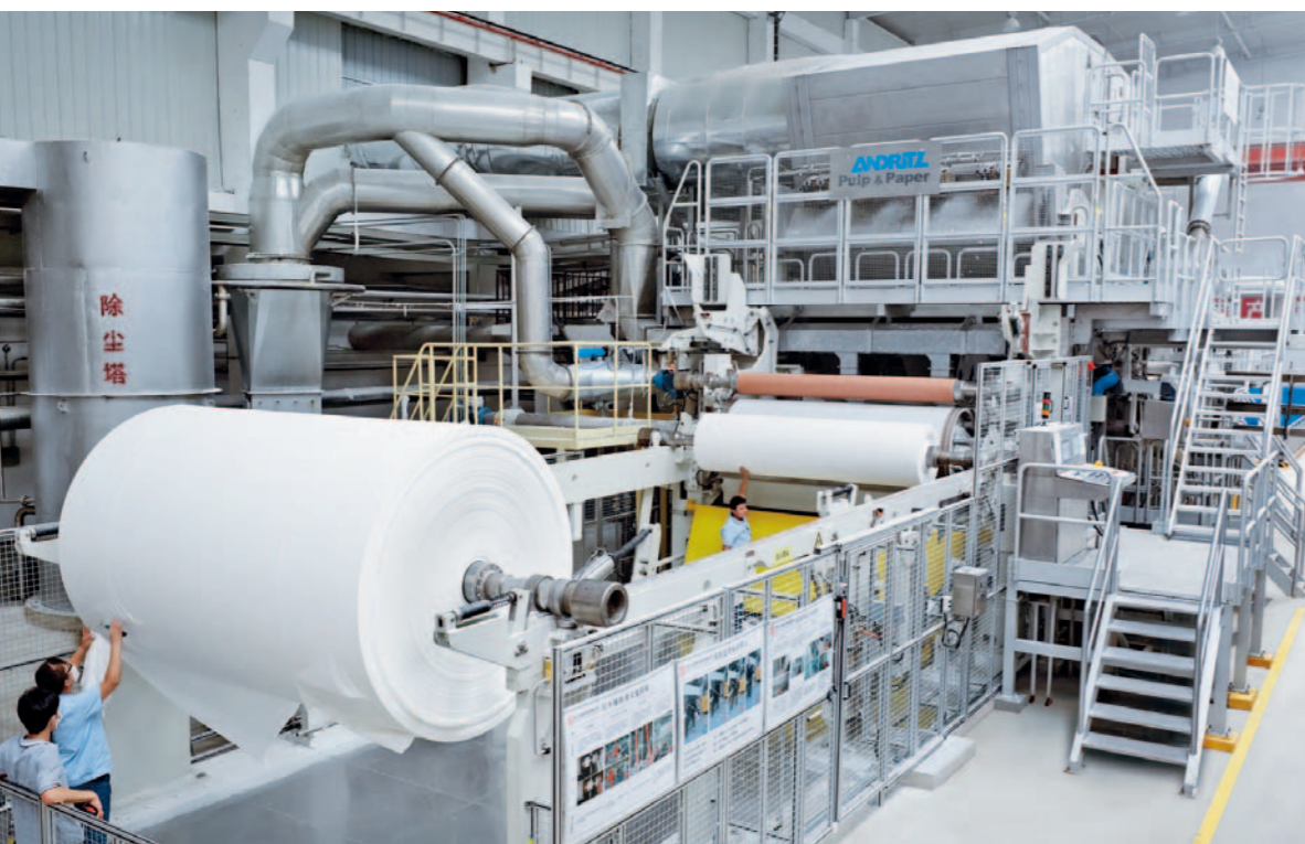
▼ PrimeLineCOMPACT tissue machine with tissue on the reel.
