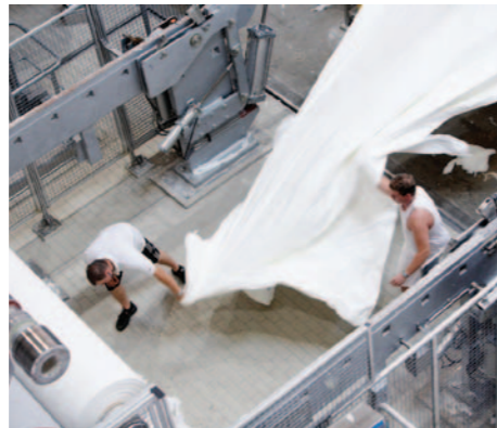
◀ Wire and felt changes can be accomplished quickly due to the modular, compact machine design.
